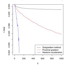
Note: accelerated proximal gradient is not a descent method ("Nesterov ripples")
