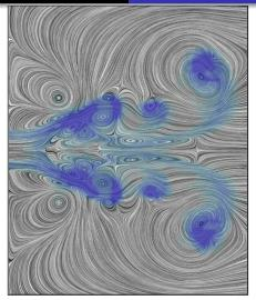
Numerical simulation of fluid flow (flow-lines in grey) + local complexity (blue) Jänicke *et al.* (2007)
