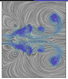
Numerical simulation of fluid flow past a cylinder (flow-lines in grey) + local complexity (blue) Jänicke *et al.* (2007)
