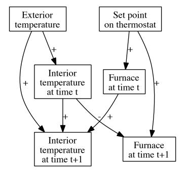
Figure 21.6: Directed, acyclic graph for the situation in Figure 21.5, taking into account the fact that it takes time to traverse a feedback loop. One should imagine this repeating to times t + 2, t + 3, etc., and extending backwards to times t - 1, t - 2, etc., as well. Notice that there are no longer any cycles.
