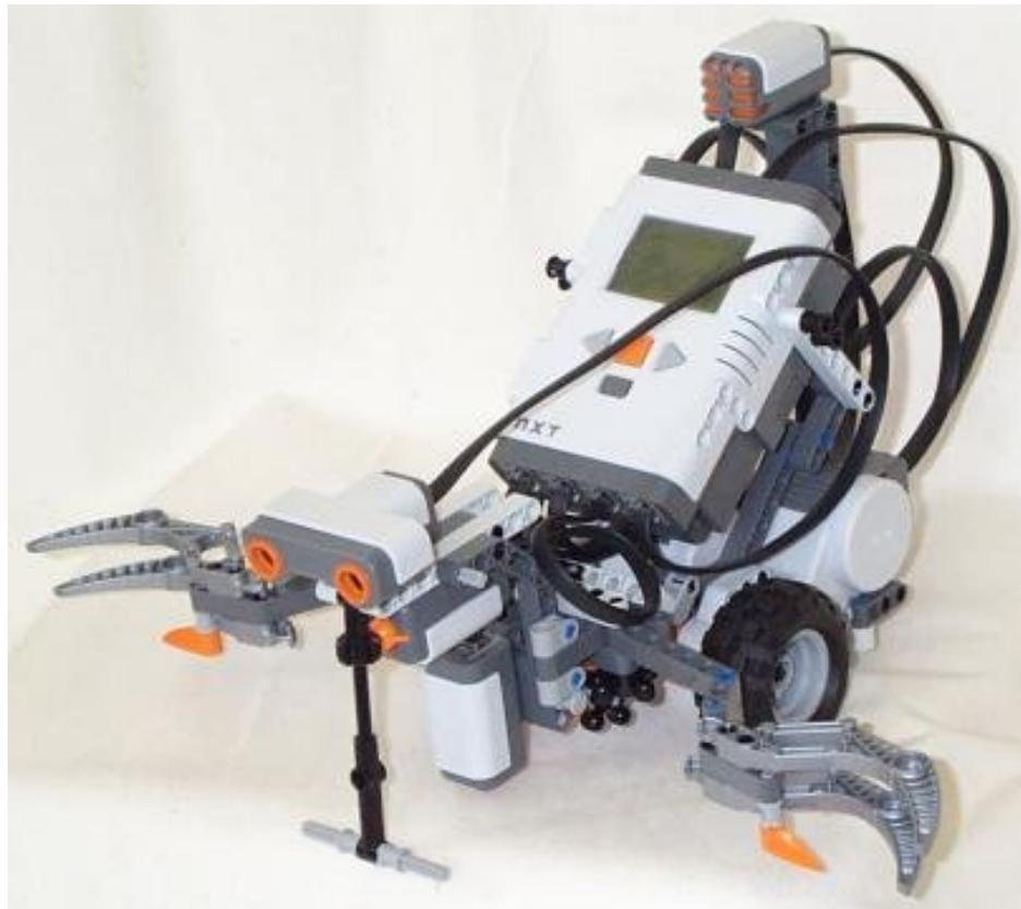
This program will wait until a ball is placed in front of the Tribot, when it will move forward until it touches the ball then stop. When you clap your hands, it will close the grabber, turn around, and return to the starting point, where it will open the grabber and drop the ball.
