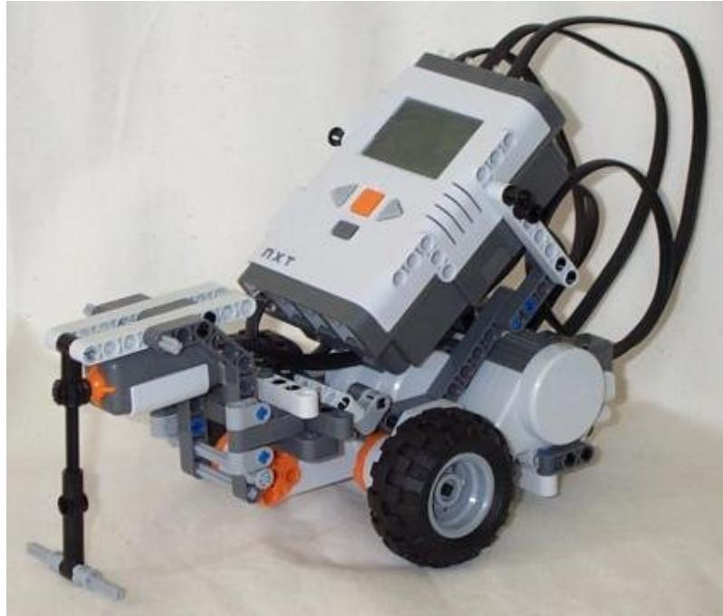
Connect the sensor to input 1 on the NXT.
