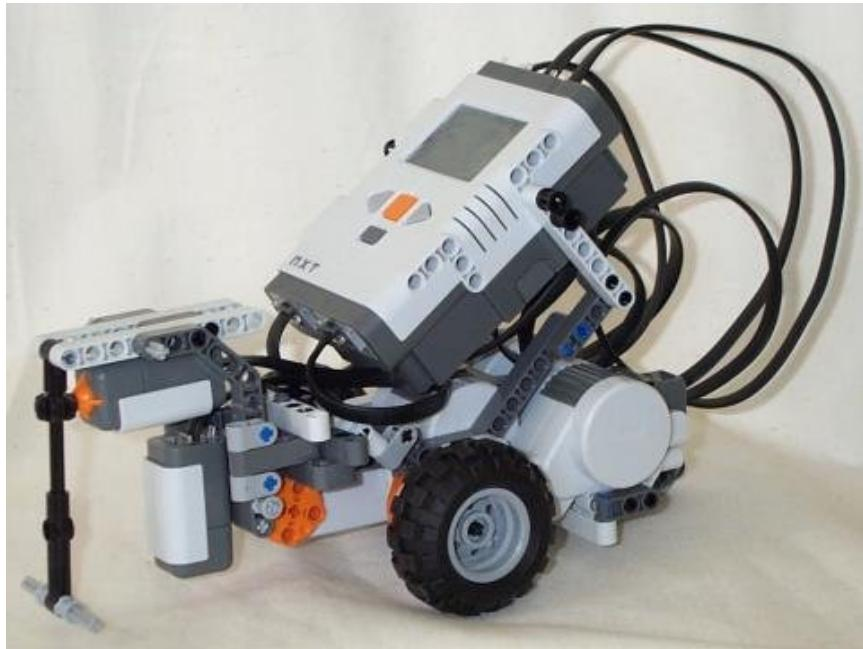
We also need the race track that comes with your NXT kit (This big piece of paper with the black track on it.) The idea now is that the robot makes sure that the light sensor stays above the track. Whenever the intensity of the light goes up, the light sensor is off the track and we need to adapt the direction. Here is a very simple program for this that only works if we travel around the track in clockwise direction.
